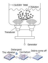
Ultrasonic cleaning is on based on the cavitation effect caused by high frequency ultrasonic wave vibration signal in the fluid. Microscopic bubbles are formed, and they implode violently causing the cavitation which create an intense scrubbing action on the surface of the item being cleaned. The bubbles are small enough to penetrate microscopic crevices, cleaning them thoroughly and consistently.
